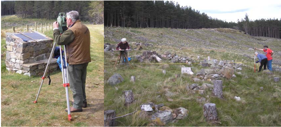
Figure 22: Volunteers undertaking Topographic (left) and Plane Table (right) survey at Druim an Aird.
