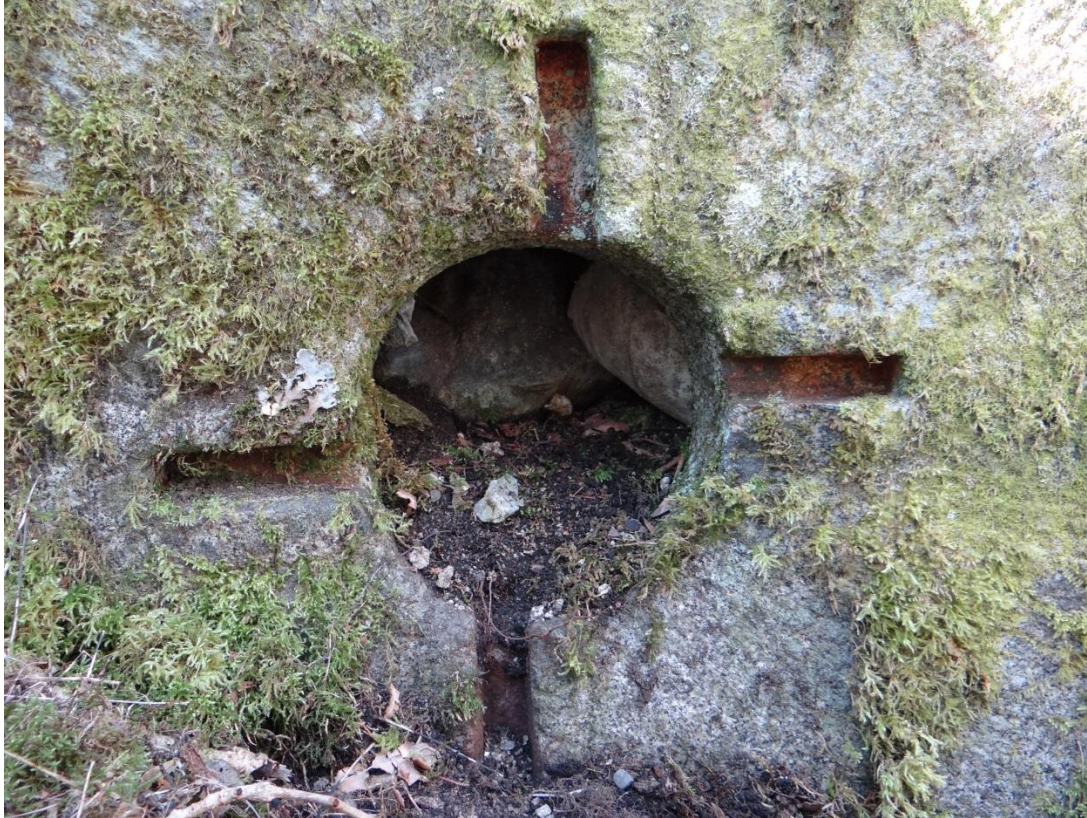
29 - Close up the centre of the mill stone showing offset rectangular sections
