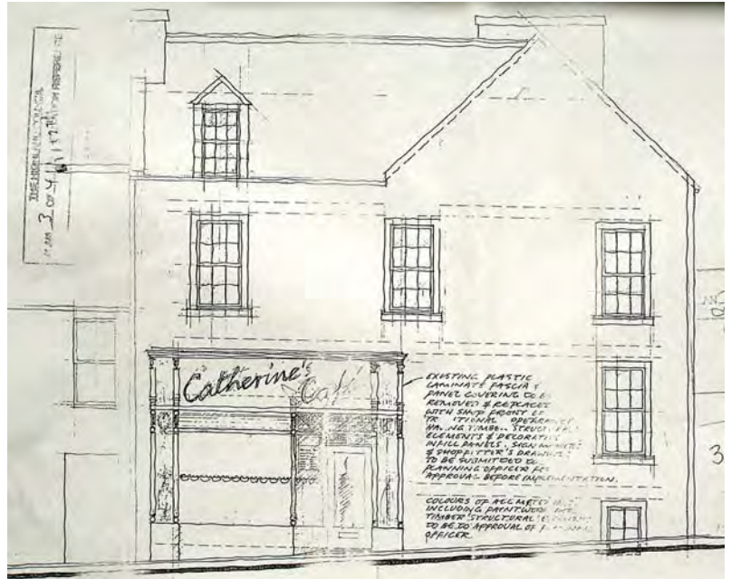
Drawing prepared by Duncan J Fraser of Inverness for the conversion of 7 Sir John's Square (1996): the elevation shows the hipped dormer remaining in position but the east chimneyhead has been removed at the gable
