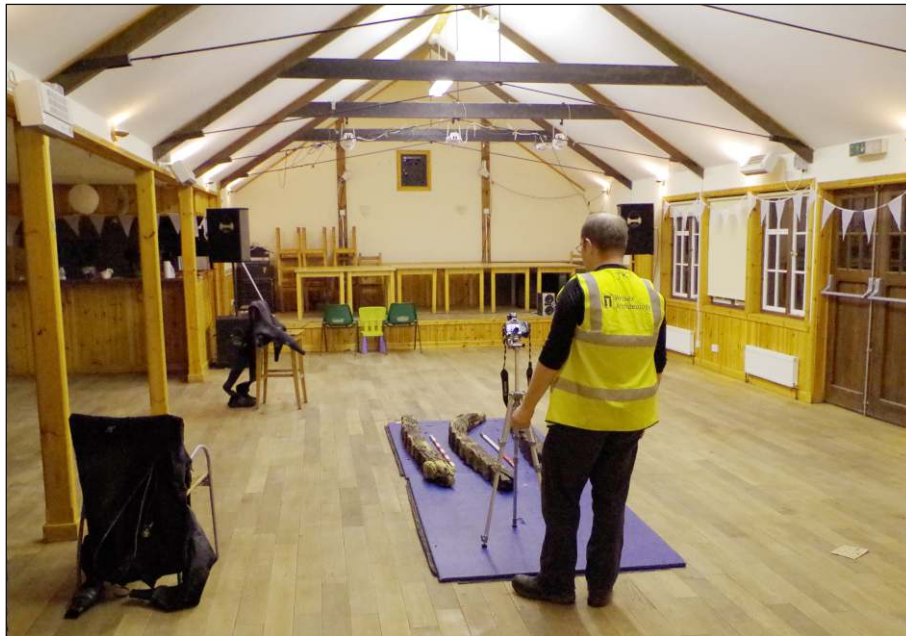
Plate 4: The photogrammetric survey of the Galmisdale timbers in the Eigg community Hall
