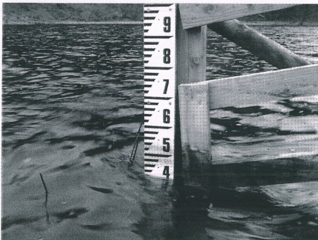
Fig.9 - Photographic Image of the in-situ Depth Gauge for the Loch, showing the reading of 420mm taken on the day of the Site Survey
